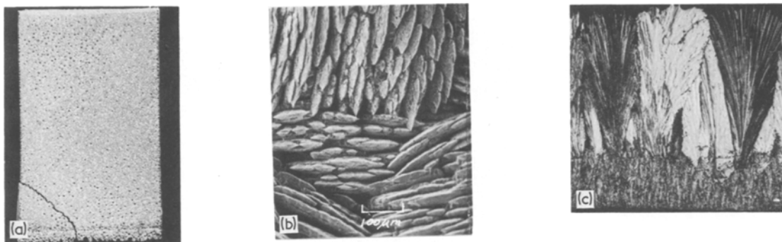
Fig. 3. Deposit from solution with 50 \text{ mg l}^{-1} glue addition: (a) Macro view, \times 0.75 ; (b) S.E.M. view of surface; (c) cross section, \times 25 .
