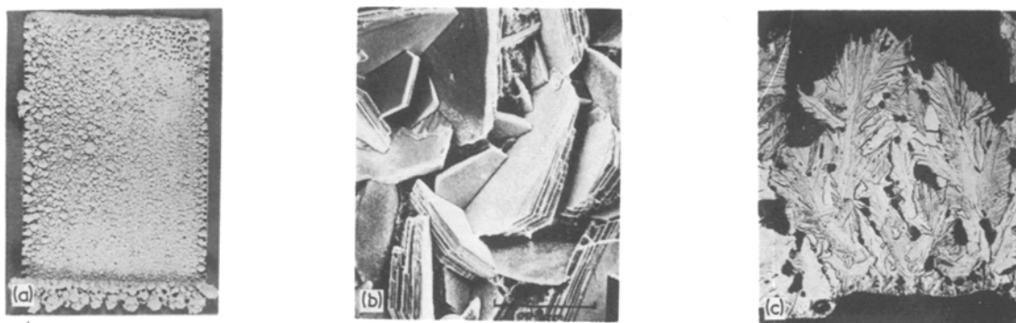
Fig. 2. Deposit from addition-free solution. (a) Macro view \times 0.75 ; (b) S.E.M. view of surface; (c) cross section, \times 25 .
